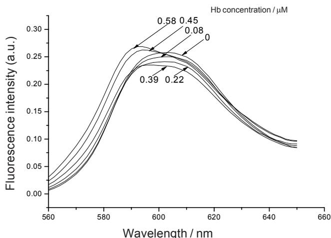
Figure 7. Fluorimetric titration of rhodamine 101 with isolated Hb-liposome complexes. Dye concentration was 3.2 nM. Lipid-to-Hb molar ratio was 440.
