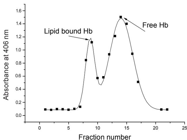
Figure 6. Elution profile of Hb-liposome mixture obtained by size-exclusion chromatography on Toyopearl HW-60F gel.
